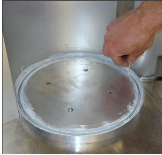
Figure 23: Ensure There is Grease in the Pail Support Groove
