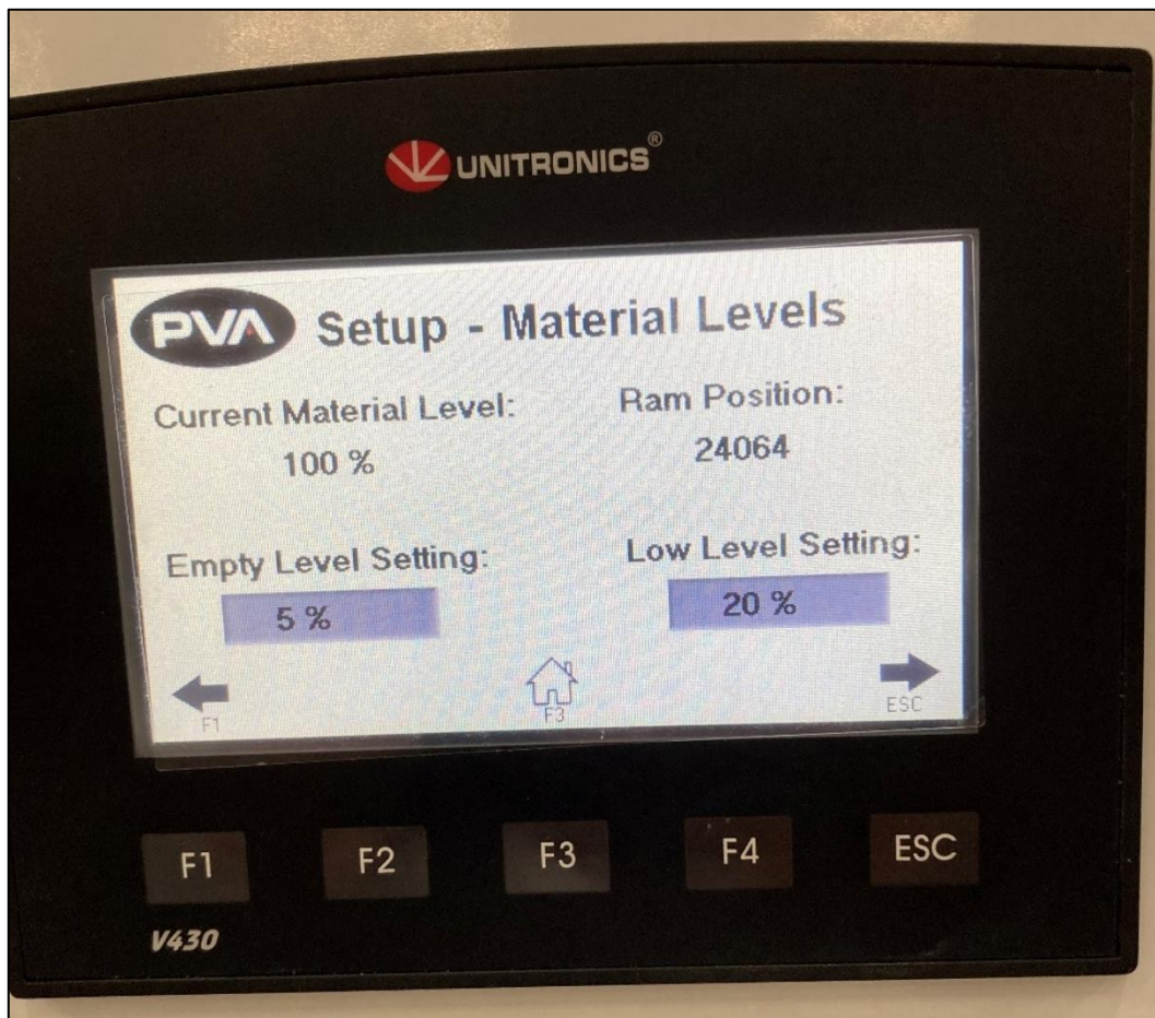
Figure 31: Setup - Material Levels Screen
