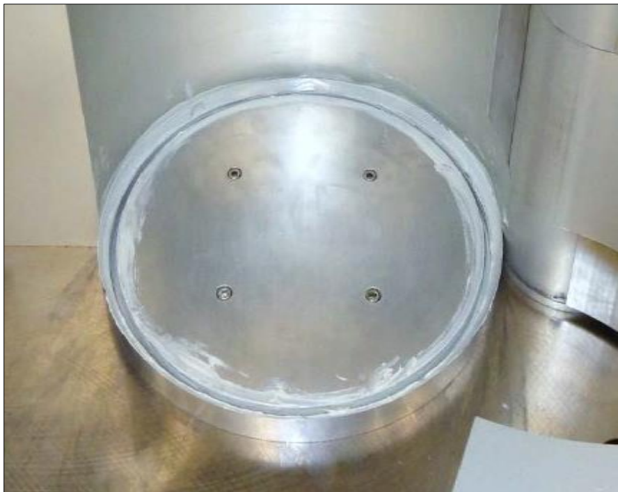
Figure 22: Apply Grease to the Pail Support Base
